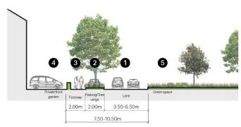
Figure 42 Section showing indicative dimensions for edge lanes. The lane width may vary to discourage speeding or provide space for parking.
